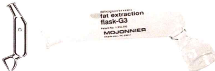
Figure 17: Mojonnier fat extraction flask. (Courtesy of Kontes Glass Co., Vineland, NJ).
