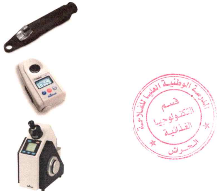
Figure. 10 Rhino Brix hand-held refractometer. R2 mini digital hand-held refractometer, and Mark III Abbe refractometer. (Courtesy of Reichert Analytical Instrument, Depew, NY.).
