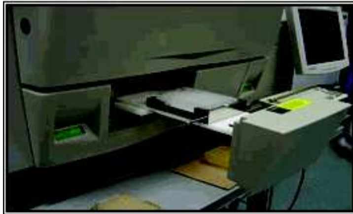
Figure 12 : The MegaBACE 3000 instrument used in our experiment.
