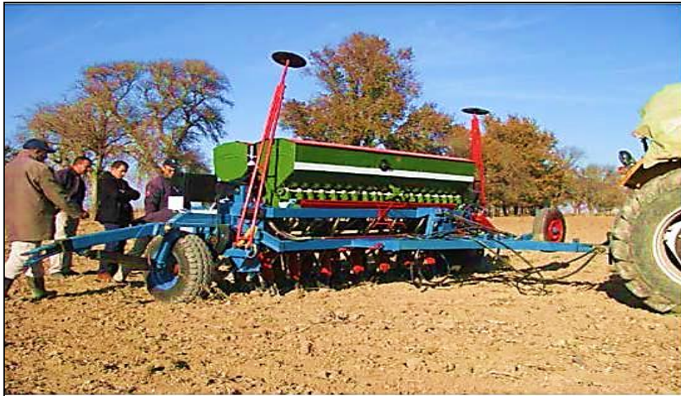
Figure 7: Semoir de semis direct Ets Refoufi ITGC Setif.
